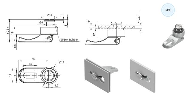
Coupling designed for joining sheets with a total thickness of 4 to 5 mm. Pressure adjustment by means of a threaded clip.
