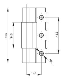
\* DIN 7985 M6 screw is not included in the scope of supply.
